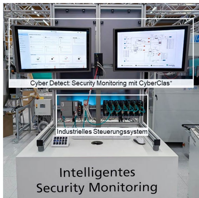
Fig. 2: The industrial test environment for evaluating the CyberClas + solution.
