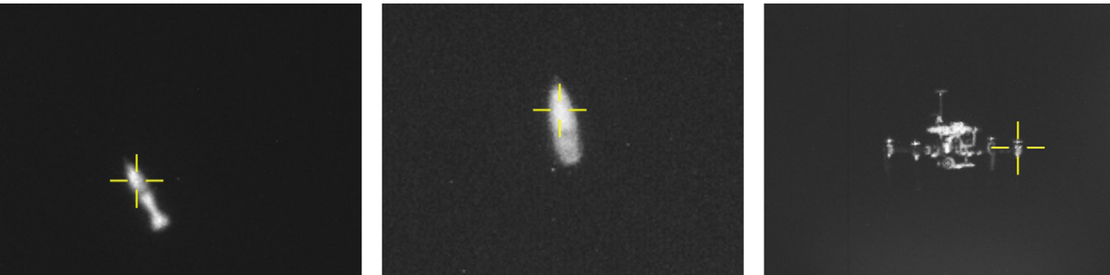
Fig. 2: SWIR Gated Viewing example images of potential targets in a HEL engagement scenario captured during measurement campaigns with the system demonstrator of Fraunhofer IOSB: 120 mm mortar (left), 155 mm artillery grenade (middle) and Unmanned Aerial Vehicle (UAV, right) with indicated aiming points generated from appropriate fine tracking algorithms.
