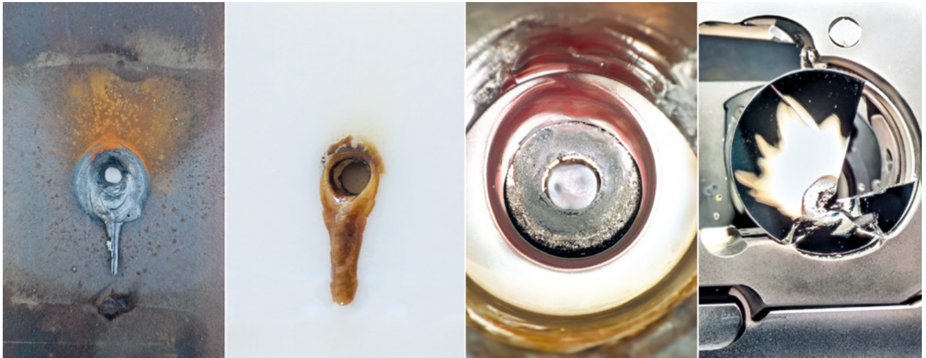
Fig. 2: Collage of laser irradiation experiments on different target materials: metal, plastic, bolometer, and mirror.
