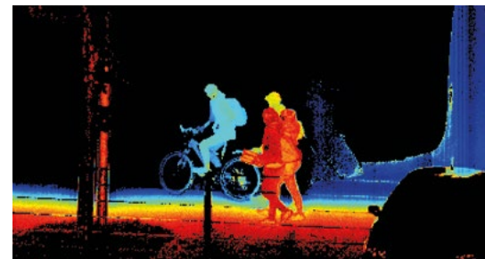
Figure 4: Color-coded range image (red-blue = 83-86 m) reconstructed from the two shown gated viewing images. The four persons can be clearly distinguished in terms of their distance.
