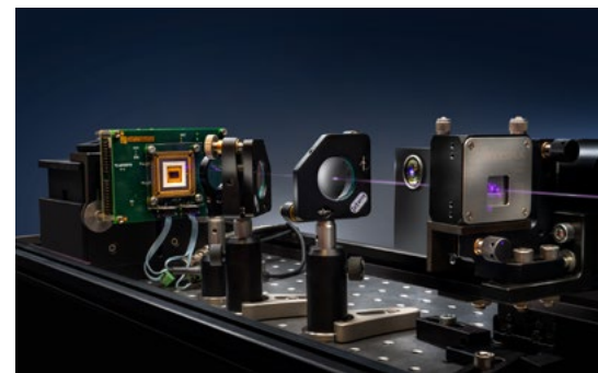
Figure 2: Quantum Light source (center) and compact single-photon detector (left)
