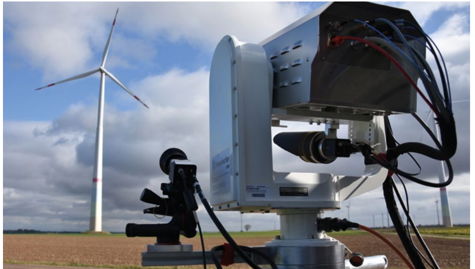
Figure 1: Head of the laser Doppler vibrometry system mounted on a pan-tilt unit together with short wave infrared cameras of the tracking system.
