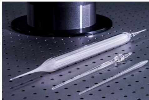
Left: Various oxide laser crystals with different active dopants (rare-earth elements and transition metals).
