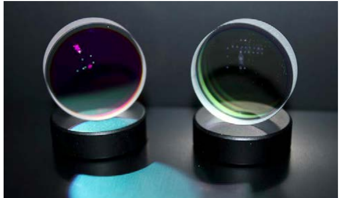
Visible damage to optical components produced and detected by the ELIDT measuring system.
