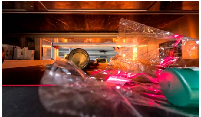
Measurement campaign for the multi-sensor collection of data from lightweight packaging waste at Fraunhofer IOSB.
