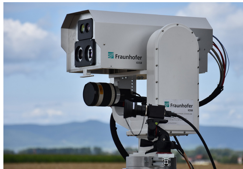
Laser Doppler vibrometer mounted on a pan-tilt unit.
