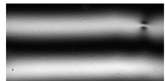
Reflection of a horizontal fringe pattern by a sheet metal sample.
