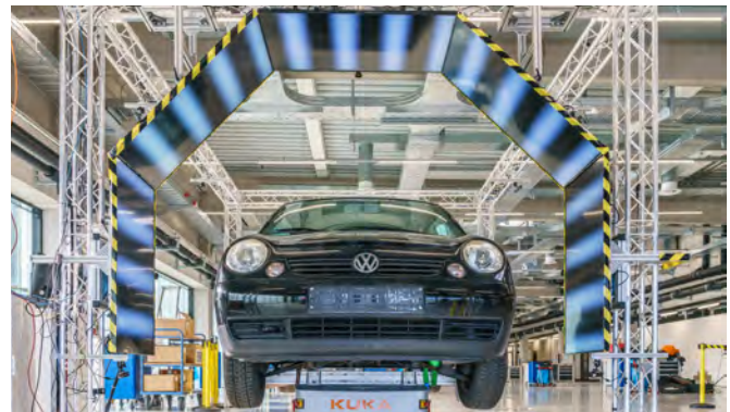
Deflectometry portal for the inspection of moving objects: Fraunhofer IOSB's AutoInspect demonstrator combines deflectometry and other inspection methods into a complete system.
