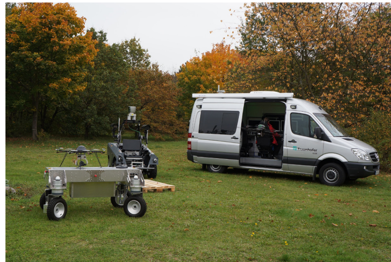
Mobile AMFIS control station (integrated in a Sprinter).
