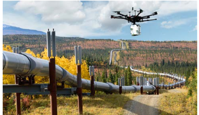
This drone and hyperspectral camera succeeded in detecting oil reliably in the test scenario.
