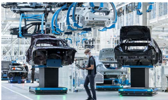
Flexible, digitized production at Mercedes-Benz: In the TecLines, classic assembly lines are replaced by automated vehicles.
