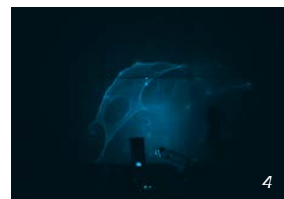
Time-dependent reflection characteristics of a near-infrared laser beam after hitting a metallic target. Initially, there is a geometrically confined reflection in a defined direction (1). Then, ring structures can emerge due to physical stress on the target (2) and when the target starts to melt, pronounced caustics form in the reflection pattern (3-4).
