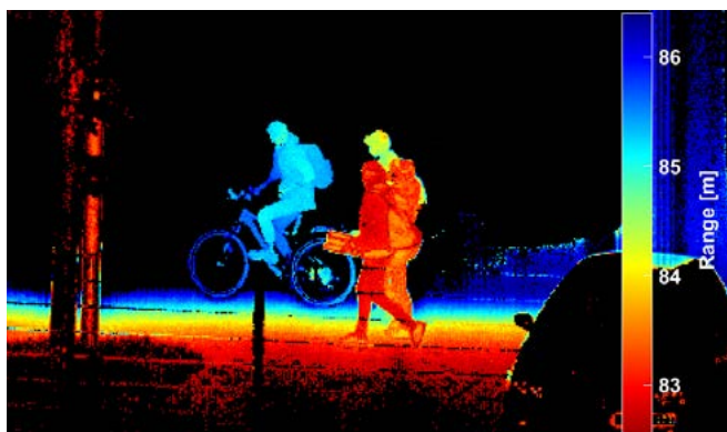
3D-GV recording of a dynamic scene with high depth resolution.
