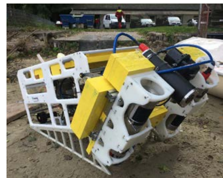
ROV belonging to UWR with integrated SeaVision laser scanner shortly before it was deployed in the Arendsee lake (November 2020).
