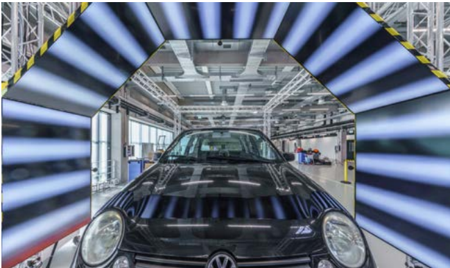
Deflectometry makes it possible to detect even minute dents or scratches in reflective surfaces.
