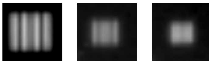
Figure 2: Test patterns as seen by an under sampled thermal imager with four, three, and two bars visible (from left).
